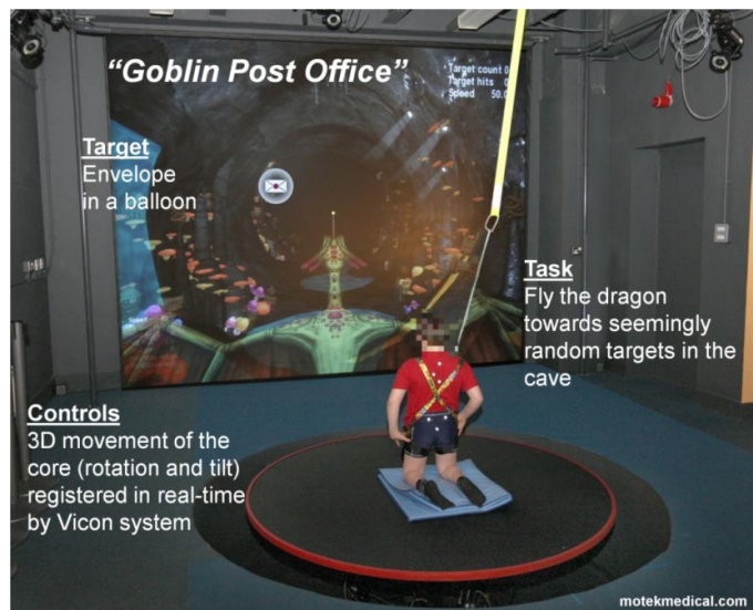
Figure 1: The Goblin Post Office game as played by the participant. Note the infra-red cameras mounted on the walls, tracking positions of the two marker clusters on the trunk and pelvis.
